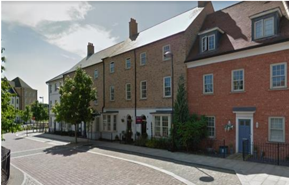
Figure 8: example pic showing use of materials to delineate parking bays
