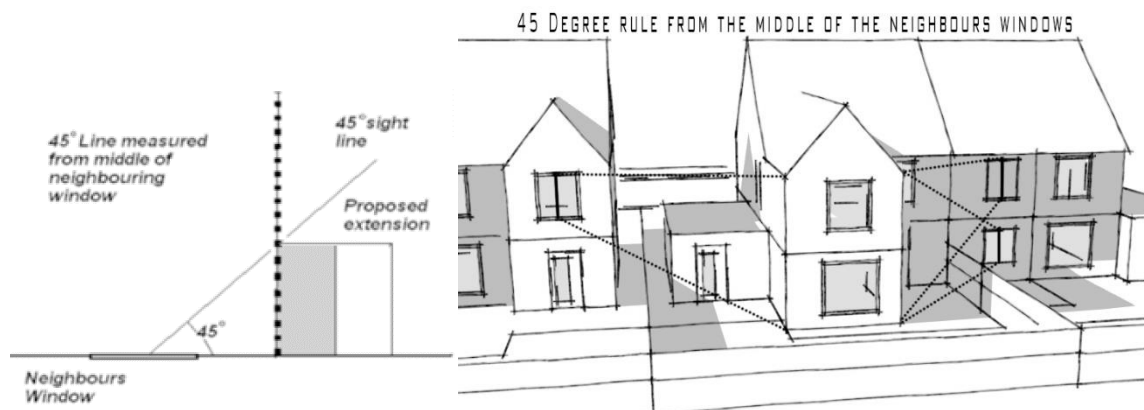
Figure 26: diagram to illustrate the 45 degree rule
